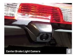
Whether reversing, driving or parking, this fully integrated, multi-camera solution provides excellent blind spot assistance. Built with trailering in mind, the three-camera system (with optional fourth camera) and user interface integrates seamlessly into your vehicle's in-dash screen.
