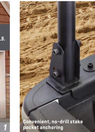
Convenient, no-drill stake pocket anchoring
