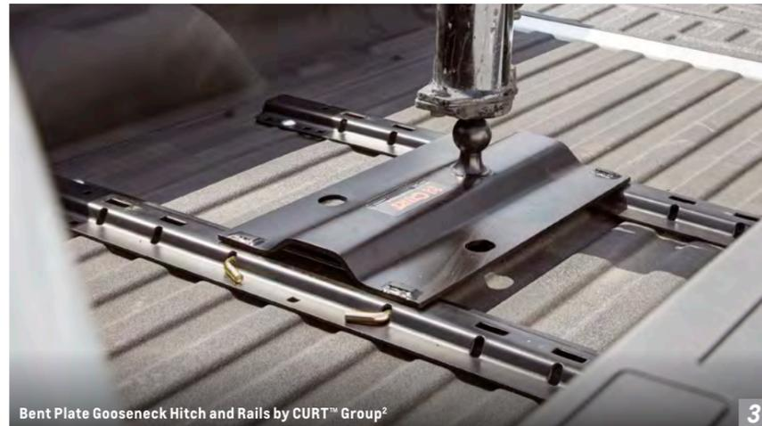
Bent Plate Gooseneck Hitch and Rails by CURT™ Group²
